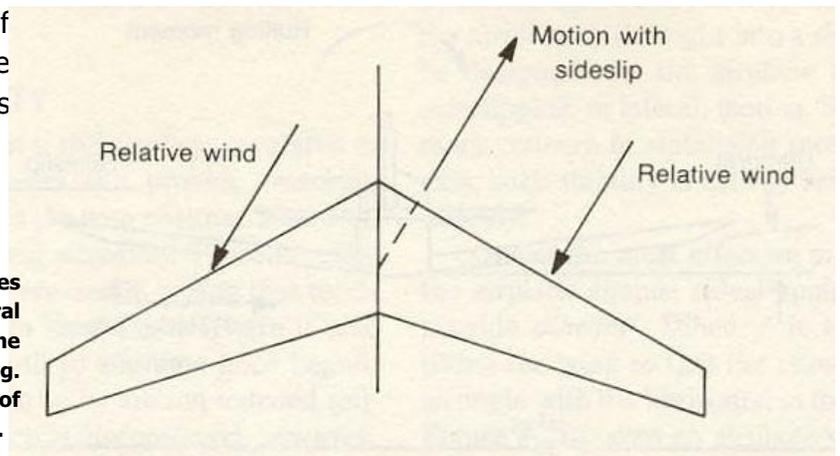
**When a swept wing yaws, the upwind panel generates greater drag and greater lift due to a difference in lateral airflow of the panels. The difference in drag resists the yaw, but the difference in lift tries to roll the wing. Depending on the wing design, three to ten degrees of sweepback are the equivalent of one degree of dihedral.**
