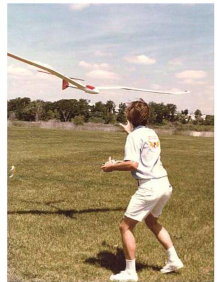
The gull wing of the author's Borne Free aileronless sailplane raises the center of lift above the center of gravity to increase pendulum stability - a desirable form of lateral stability, especially when circling in a thermal. Inboard panels of the wing add to the side area to resist side slip.
