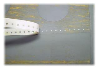
Pop rivets have a hole in their centers. If the glue is diluted even more and just right, it will wrinkle slightly when drying, creating a pop-rivet look. This requires some experimentation to get right—try it on a scrap surface first. Rivet tape can be reused but only once or twice.
