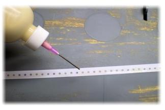
Attach the rivet tape. Apply a 20% diluted solution of white or yellow glue. For flush rivets, squeegee off the excess with a credit card. For domed rivets, place a drop of glue over each hole and don't squeegee. Remove the tape immediately while the glue is wet. The rivets will appear to be too large at first but they will shrink as the glue sets.
