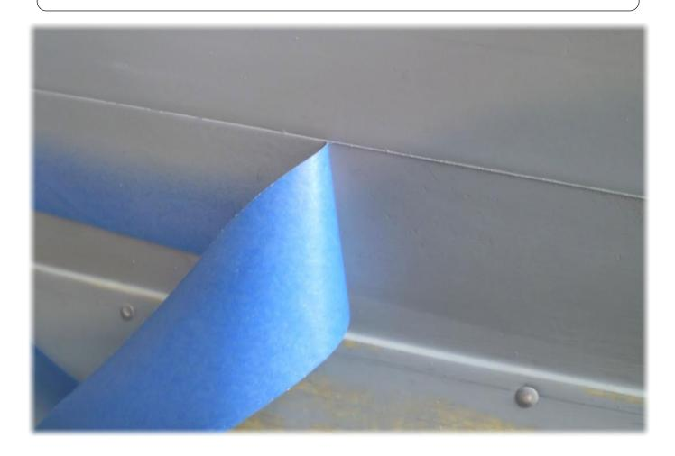
Sometimes prominent hatches such as gun covers require a surface too thick to be implemented with primer. In this case, mask off the hatch with more than one layer of masking tape, apply a thin layer of Bondo or other automobile body putty with a squeegee or credit card and sand to the tape. Remove the tape and lightly sand the edges.
