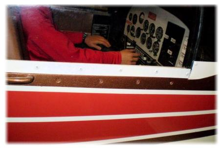
Phillips pan-head and flathead screws appear on the Grumman Lynx and other modern airplanes. The best way to simulate screw heads is to use real screws. Miniature screws in a large variety of styles and sizes are available from MicroFasteners.
