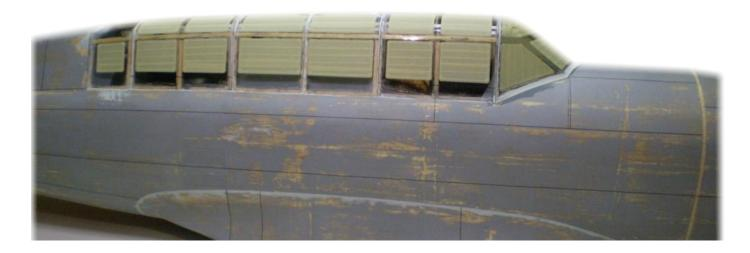
Apply another coat of primer with a mini-roller. Sand off almost all of it, leaving the Chartpak tape exposed.
