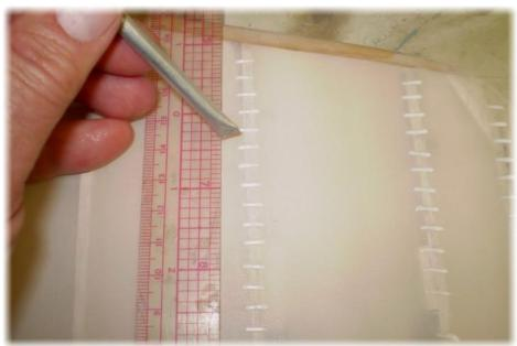
Scotch Hair Set tape is about right for quarter scale. Apply it or other pinking tape (see Ref) over the rib stitches. Apply nitrate dope to Scotch Hair Set tape to secure the tape and to raise the fibers. Sand smooth.
