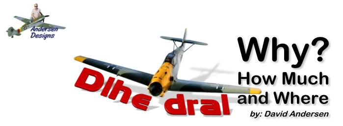
Dihedral is the upward angle of an aircraft's wings. It increases stability in roll, also known as lateral stability. Some airplanes need a lot, others need less or none or even negative dihedral.
