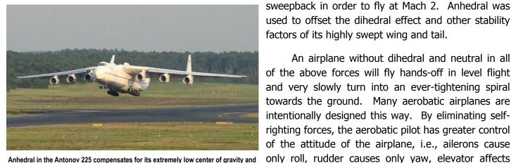
Anhedral in the Antonov 225 compensates for its extremely low center of gravity and reduces unwanted yaw and roll in the event of engine failure.
