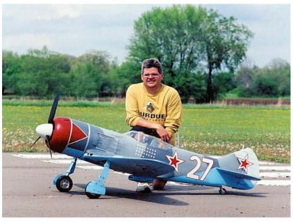
Jeff Quesenberry's Lavochkin La 7 displays the modest dihedral typical of WW2 single-engine fighters—just enough for hands-off stability during long flights but not enough to interfere with fighter aerobatics or gun aiming or to cause Dutch roll at high speed.
