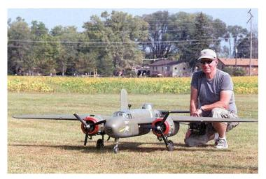
Richard Steine's B-25 has no dihedral in its outer wing panels. Unwanted yaw and roll are minimized if one engine fails. Mid-wing configuration plus inboard dihedral raises the center of lift above the center of gravity, producing pendulum stability - a brilliant balance of compromises. Appearance of negative dihedral is an optical illusion.
