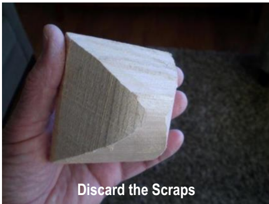
Round the edges with a razor plane and sand smooth
