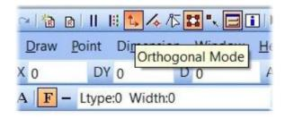
Click on the orange square with the two red arrows labeled "Orthogonal Mode". This causes all lines that we draw to be either horizontal or vertical-what we need for drawing dimensions.
