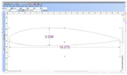
It might be necessary to click on "View" and "Fit to Window" if the result is too big or too small for the window. It might also be necessary to zoom in on part of the drawing in order to make tiny movements of the handles. If so, click on "View" and click on "Zoom".
