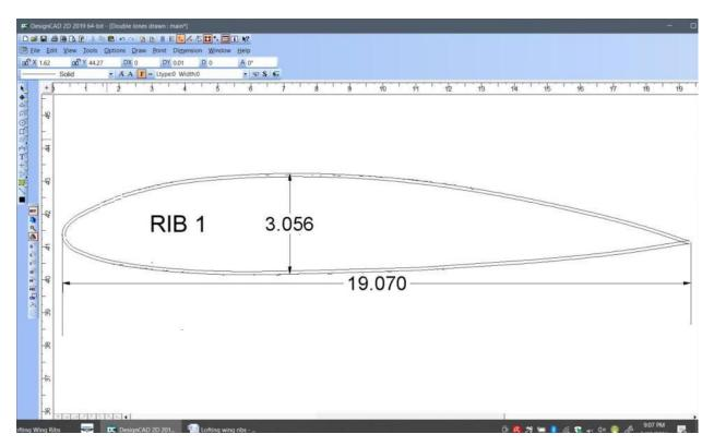
Move the cursor (and the text) to where you wish to have it displayed and double click. The text will be written as bolder print on the drawing. Save the drawing ("File"--Save As...") for later reference with the file name "Rib 1" or something similar.
