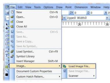
Move the cursor to the upper left and click on "File". Move the cursor down to "Image..." and right to click on "Load Image File...". Select the file containing the scanned airfoil JPG image and click on it.
