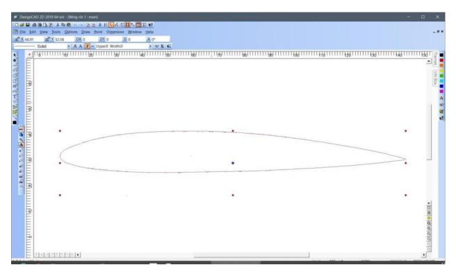
A new fine-line image of the airfoil will appear that is DesignCAD's representation of your airfoil. If you click on various parts of the image, changes in color will show that it consists of several short line segments. Again, handles appear at the edges of the image.
