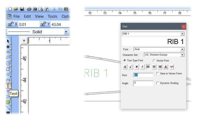
Lets add a title to the drawing. Click on the T (for TEXT) on the left side of the screen. A "Text" window will appear. Enter the text, e.g., "RIB1" and the text "Size" e.g., 0.5. "RIB 1" will appear in the drawing as light characters. The cursor will appear on the text.
