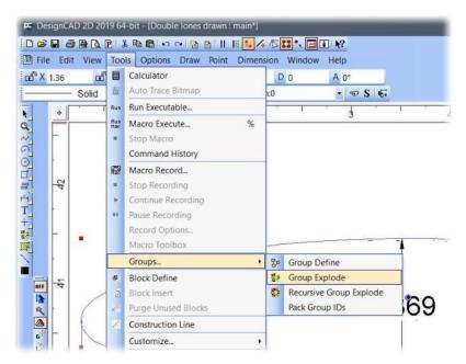
Click on "Tools", scroll down and click on "Group Explode". This breaks the drawing into separate pieces so that we can redefine the group. Click on "Edit" and click on "Select All" to combine all segments of the drawing. This allows us to "drag and drop" the handles to change the chord and height of the airfoil.
