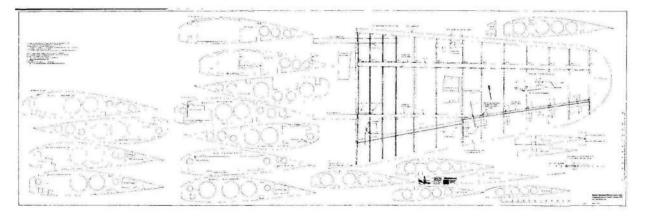
This technique can also be used for drawing horizontal and vertical stabilizer ribs. The method can also be adapted to lofting fuselage formers. Consider using the rotate command (Edit—Selection Edit—Rotate) to twist ribs for washout.
