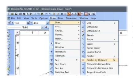
Next, we draw an inside line parallel to the airfoil that is the thickness of the wing sheeting, e.g. 3/32" =0.09375". Click on "Draw", over to "Line" and down to click on "Parallel by Distance".
