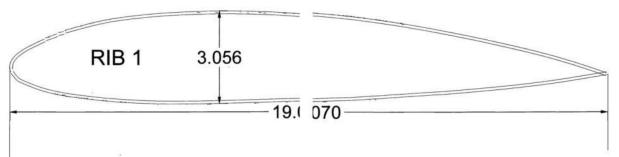
In this example, Rib1 will be printed on two sheets. Each sheet will have a mark in each corner. Load your printer with vellum paper and print. Assemble the two sheets so the corner marks align and tape the two sheets together.
