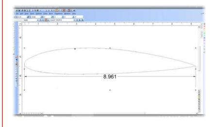
Move the cursor to the left vertical line and click once. Move the cursor to the right vertical line and double click. A horizontal dimension line with arrowheads will appear with the distance between the vertical lines displayed.
