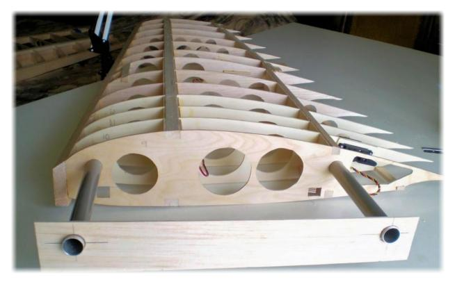
To begin, draw the plan for the wing and measure the chord of the wing at each rib location. Also draw a front view of the wing and measure the thickness of the wing at each rib location.
