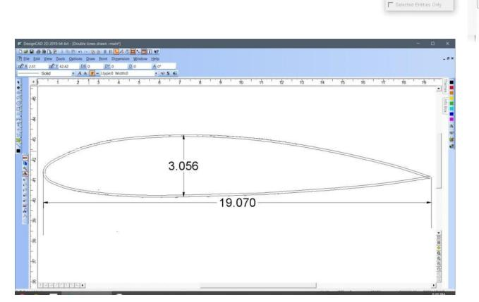
A parallel line will appear. If you move the cursor outside the line a parallel line will appear outside the line. If you move the cursor inside the line the parallel line will move inside the line. Move it inside and click. A parallel line will be drawn inside the airfoil line. The airfoil consists of several connected lines, so you must repeat this process all around the airfoil.
