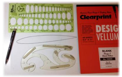
Trace the outline of the airfoil from the airplanes 3-views. Use translucent vellum paper and a fine-point pencil or pen. Use an ellipse drawing template to trace the leading edge and a French curve for the remainder of the airfoil. These tools are available at artist supply stores.
